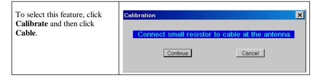
Disconnect the coax from the antenna. Then connect a small resistor in the range of 20 to 100 ohms at the antenna end of the coax. The actual value is not critical as long as you can measure it accurately with a digital ohmmeter. The resistor can be a ¼ watt size since it doesn't have to handle any power. Click "continue" after the resistor is in place.
