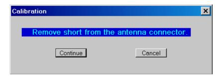
**Replace** the short circuit with an **open connector** (included with the AIM4170) and then click **Continue**.
