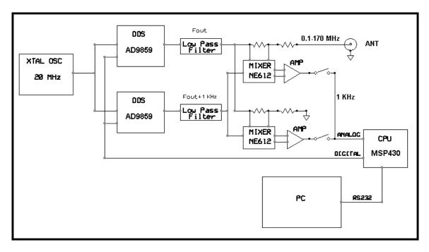
The AIM4170 uses two Direct Digital Synthesizer (DDS) chips. One generates the test signal and the other acts as a local oscillator to heterodyne the RF signals to the audio range. You can read about the basic principles of the DDS at this address: <a href="http://www.analog.com/library/analogDialogue/archives/38-08/dds.pdf">http://www.analog.com/library/analogDialogue/archives/38-08/dds.pdf</a>
