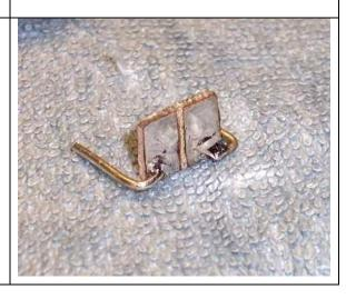
Here we see the surface mount adapter combined with the binding post adapter. The stray capacitance of this combination adapter will also be compensated by the calibration procedure. Capacitors in the picofarad to nanofarad range and inductors in the nanohenry to microhenry range can be measured.
