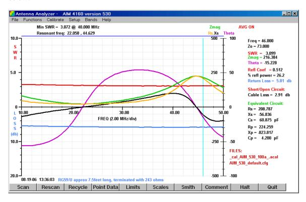
The light cyan vertical line is the cursor. It moves with the mouse whenever the mouse pointer is inside the graph area. In this example, the frequency is 46.000 MHz. The frequency changes in 1-pixel increments due to the mouse resolution, so some specific frequencies may not be displayable. The data is interpolated between the actual data points that were recorded during the scan. The cursor can also be moved in small increments using the Left/Right Arrow Keys on the keyboard.
