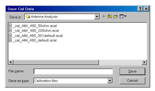
Enter the name of the calibration file and click "Save". There is no restriction on the name of the cal data file. It's extension is automatically set to .acal ("analyzer cal"). Any of these cal files can be recalled latter using the menu option "File" → Load Cal File.
