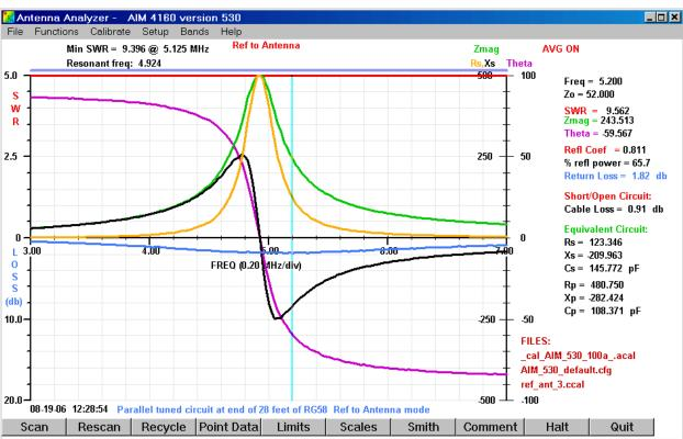
The cursor data at 5.200 MHz is very close for both plots. To exit from this mode, click "Functions" and "Ref to Antenna" again.
