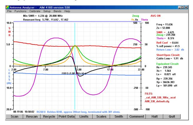
This picture shows an **ordinary** scan with a 301-ohm resistor at the end of 28 feet of RG58 coax. The Green trace is the magnitude of the measured impedance. As expected, this is a complex function of frequency. The magnitude of the impedance at the half-wavelength frequency is only 239 ohms instead of the expected 301 ohms because of loss in the cable.
