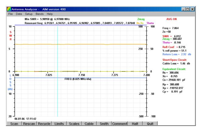
Scan using a 301 ohm resistor for a test load.
