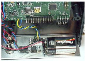
In the lower left corner of the board are shown the pos(+ RED) and neg(- BLUE) battery connections.
