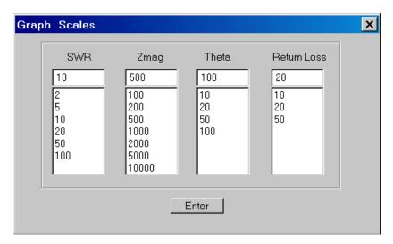
If the actual measured value is off the scale (flat line at the top of the graph), the value readout by the cursor is still valid since it uses the raw data stored in memory. For example, you can set the Zmag scale to 500 ohms in order to see fine details but if the impedance actually goes up to 1600 ohms at some frequencies, the cursor can still read the true value and display it in the data window.
