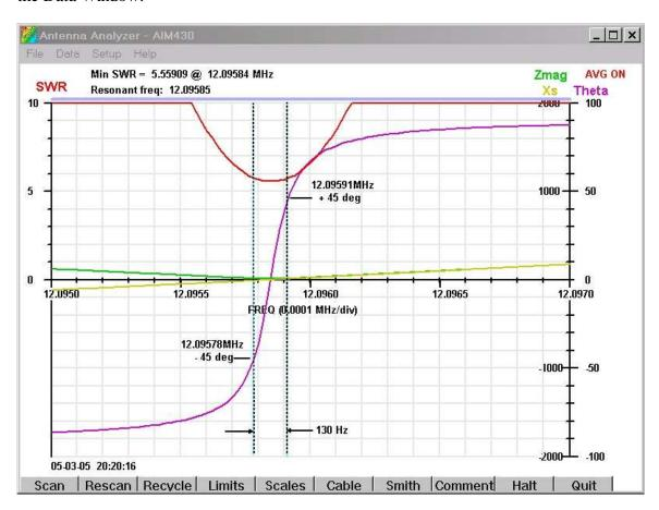
At frequencies well below the series resonant point, the impedance value is the total capacitance, Ctotal, which is essentially equal to Cparallel.
