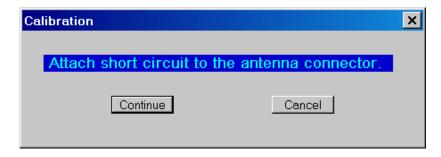
Attach the BNC connector with an internal short circuit (this is included with the AIM4170, it is labeled "short").
