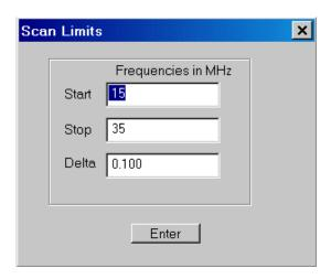
For example, to scan the 40-meter band, you might enter 6.9MHz for the Start frequency, 7.4MHz for the Stop frequency and 0.01MHz for the frequency Step (the spacing between measured points). This would result in a scan of 50 points across the band. The maximum number of scan points is 300 and the minimum number is 5.
