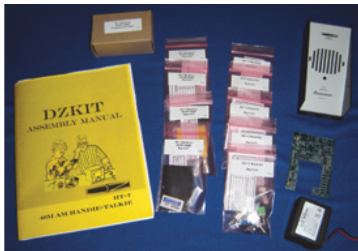
Figure 5 —The HT-7 kit pieces are well packed and organized. Surface mounted components are already soldered to the PC board.
