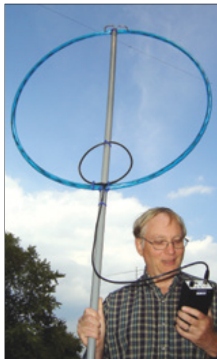
Figure 8 — Fellow ARRL Lab Engineer Mike Gruber, W1MG, with the HT-7 and portable loop antenna.
