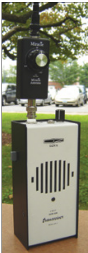
Figure 7 — Here's the finished HT-7 with its optional Miracle Antenna tuner and whip.
